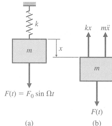
$$x(t) = X \sin(\omega t + \varphi) + \frac{F_0/k}{1 - (\Omega/\omega)^2} \sin \Omega t$$
