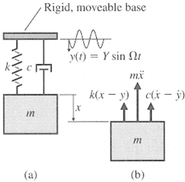
$$\begin{aligned}m\ddot{x} + c\dot{x} + kx &= ky + c\dot{y} \\m\ddot{x} + c\dot{x} + kx &= kY \sin \Omega t + c\Omega Y \cos \Omega t \\m\ddot{x} + c\dot{x} + kx &= Y \sqrt{k^2 + (c\Omega)^2} \sin(\Omega t - \gamma) \\\gamma &= \tan^{-1}\left(-\frac{c\Omega}{k}\right) = \tan^{-1}(-2\xi r)\end{aligned}$$
