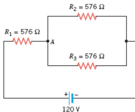
**70. REASONING** The power  $P$  dissipated in each resistance  $R$  is given by Equation 20.6b as  $P = I^2 R$ , where  $I$  is the current. This means that we need to determine the current in each resistor in order to calculate the power. The current in  $R_1$  is the same as the current in the equivalent resistance for the circuit. Since  $R_2$  and  $R_3$  are in parallel and equal, the current in  $R_1$  splits into two equal parts at the junction A in the circuit.
