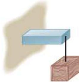
57. **REASONING** The shear stress is equal to the magnitude of the shearing force exerted on the bar divided by the cross sectional area of the bar. The vertical deflection  $\Delta Y$  of the right end of the bar is given by Equation 10.18 [ $F = S(\Delta Y/L_0)A$ ].
