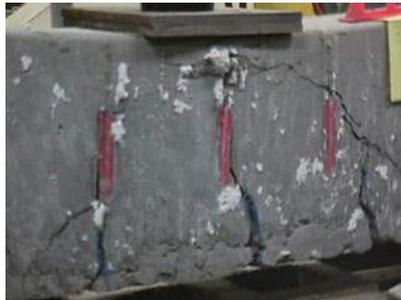
Fig. 14: Fracture of the concrete beam
