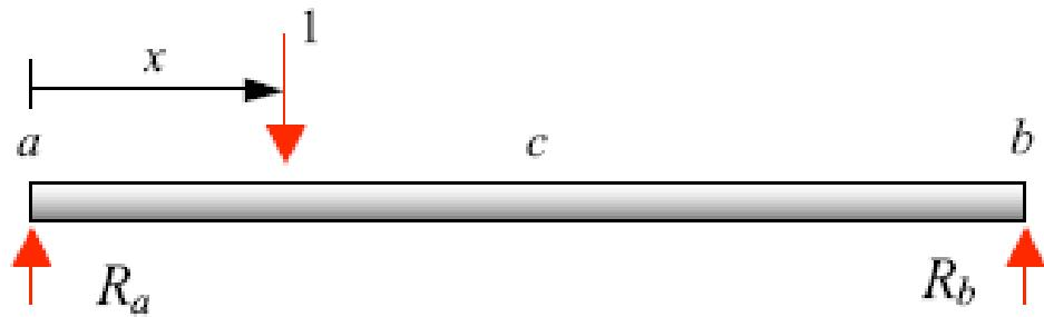
$$\Sigma M_b = 0 \quad \Rightarrow \quad R_a = (L-x)/L$$
