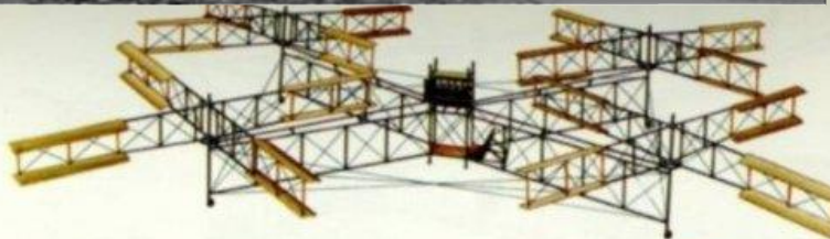
2 Paul Cornu helicopter, November 1907. Engine: One 24 h.p. Antoinette piston-engine. Rotor diameter (each): 19 ft. 8½ in. (6-00 m.). Length: approx. 20 ft. 4½ in. (6-20 m.). Empty weight: 419 lb. (190 kg.). Take-off weight: 573 lb. (260 kg.).
