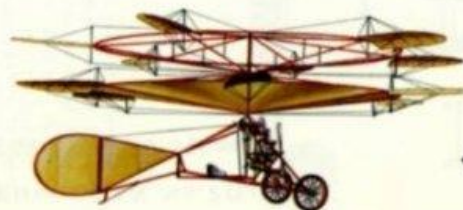
3 Ellehammer helicopter of 1912. Engine: One 36 h.p. Ellehammer air-cooled radial piston-engine. Rotor diameter (each): 24 ft. 6½ in. (7-47 m.). No other details known.
