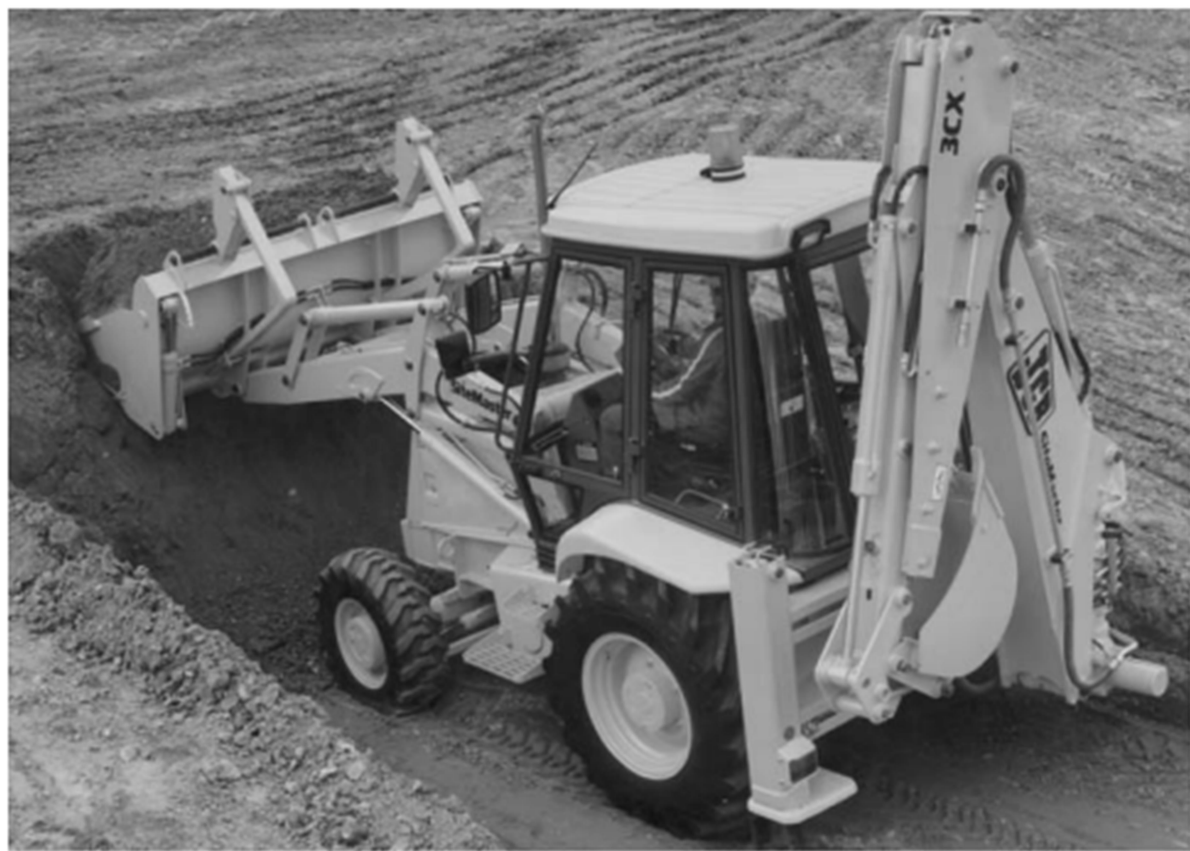
Plate 8b. The ubiquitous backhoe loader used on many sites. That shown is the JCB 3CX 56.5 kW, with shovel up to 2.3 m wide and hoe bucket 0.3–0.9 m wide. JCB Ltd, Rocester, UK
