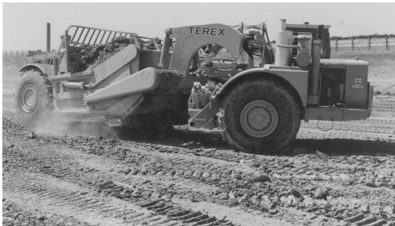
Plate 3a. A Terex TS24C 552 kW twin-engined 36 m 3 capacity scraper for earth-moving. Terex Equipment Ltd, Motherwell, Scotland
