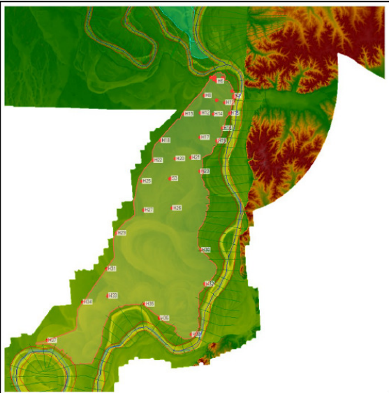
Figure 4-105. Combined One- and Two-Dimensional HEC-RAS Model of the Mississippi, Ohio, and New Madrid Floodway
