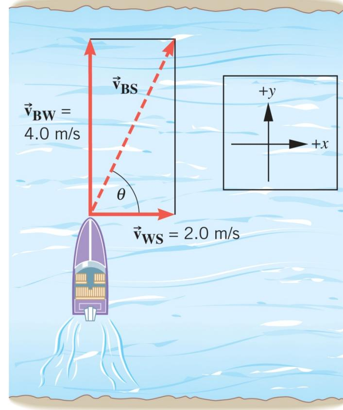
$$v_{BS} = \sqrt{v_{BW}^2 + v_{WS}^2} = \sqrt{(4,0 \text{ m/s})^2 + (2,0 \text{ m/s})^2}$$
