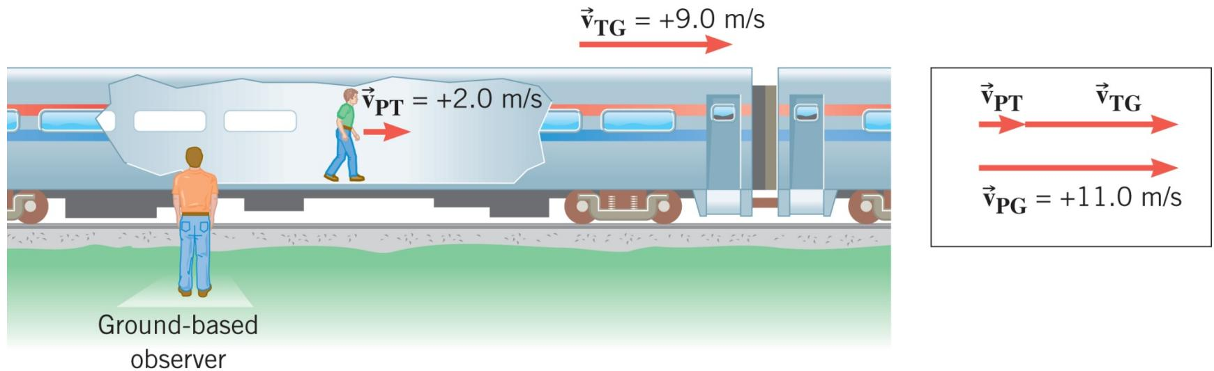
$$V_{PG} = V_{PT} + V_{TG}$$
