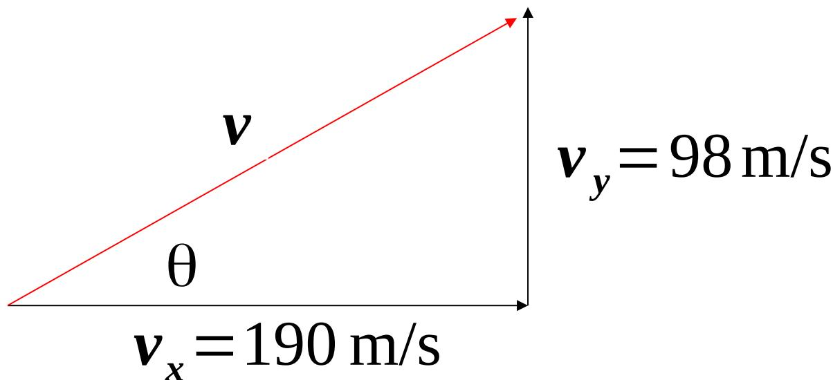
$$v = \sqrt{(190 \text{ m/s})^2 + (98 \text{ m/s})^2} = 210 \text{ m/s}$$
