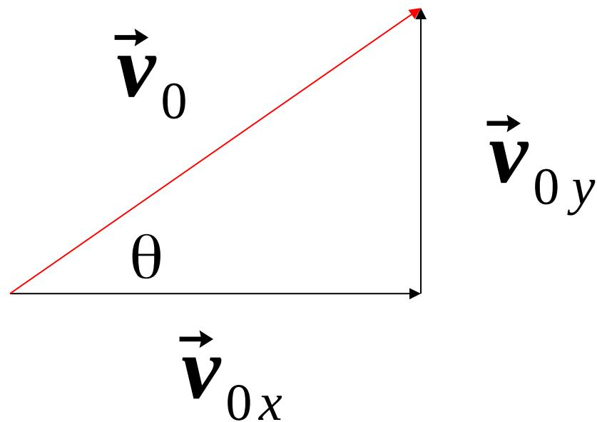
$$v_{0x} = v_0 \cos \theta = 22 \text{ m/s} \cdot \cos 40^\circ = 17 \text{ m/s}$$
