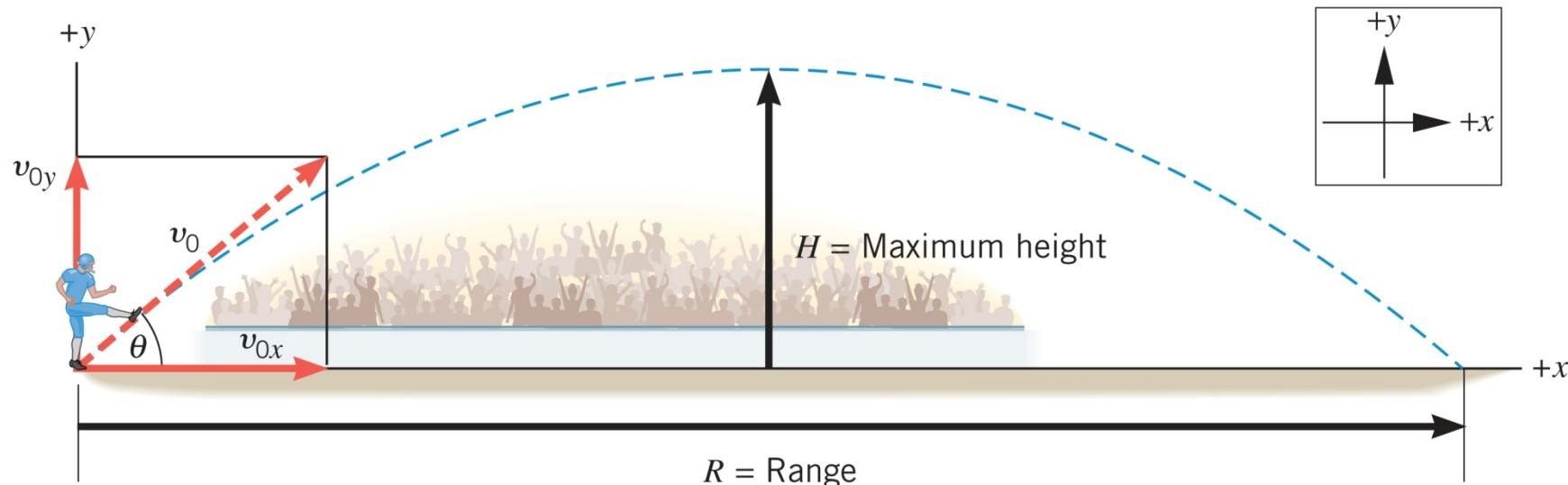
$$x = v_{0x} t + \frac{a_x}{2} t^2 = v_{0x} t$$
