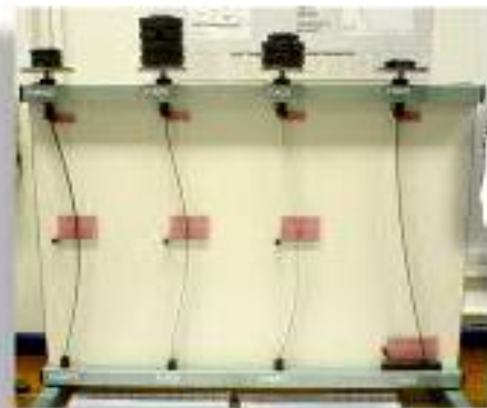
Buckling of columns
