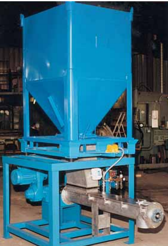
Typical industrial application: hopper discharge using external vibrator.
