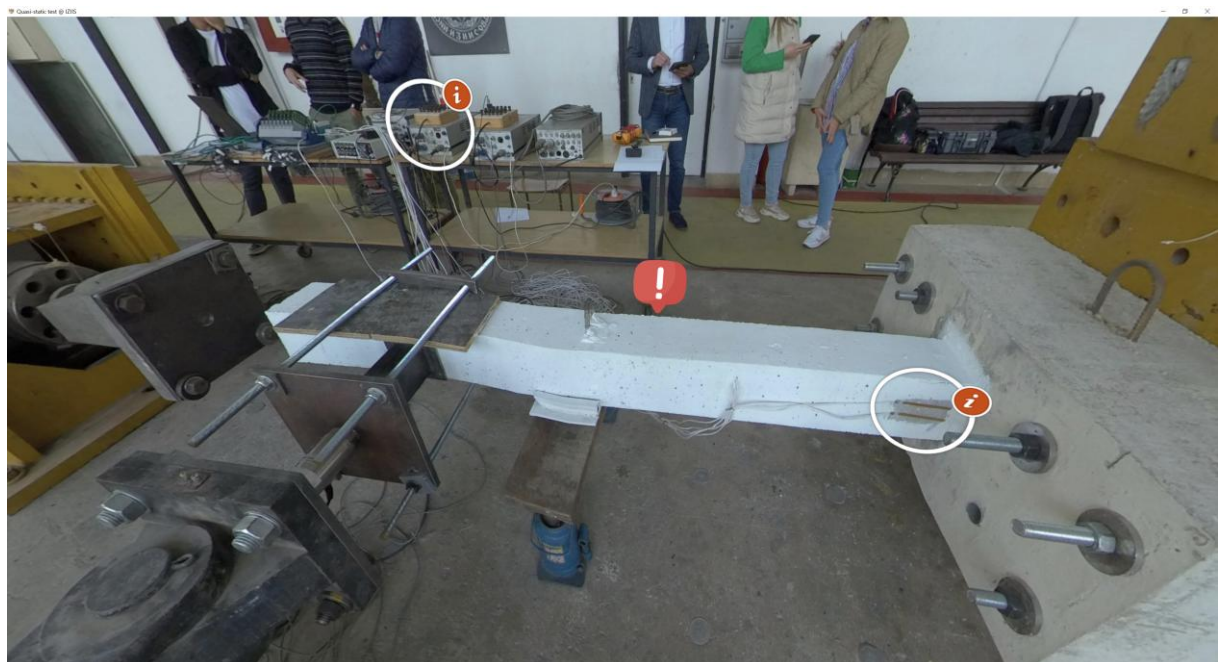
Figure 5.9: Column scene of the VT from the quasi-static test at IZIIS (before damage)
